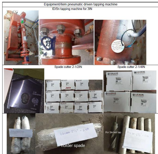
Gambar 4. Equipment Hot Tap
