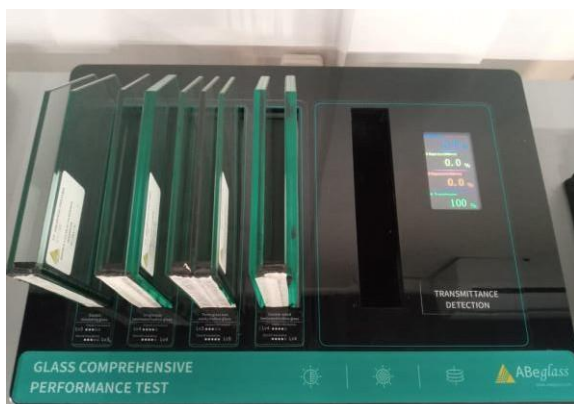
Gambar 4 . Glass Comprehensive Performance Test
