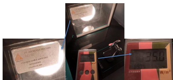
Gambar 11 . Pengujian Kaca Low E Softcoat Optitherm (Thermal Insulated Test)
