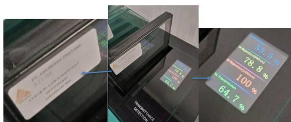
Gambar 8 . Pengujian Kaca Low E Softcoat Optitherm (Comprehensive Performance Test)
