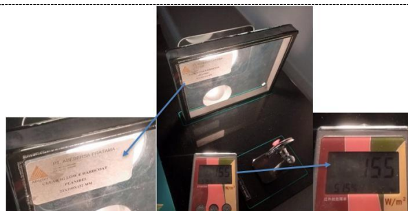
Gambar 10 . Pengujian Kaca Low E Hardcoat Planibel (Thermal Insulated Test)
