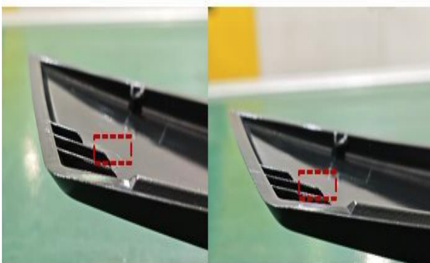
Gambar 2. Part shortmold area rib Sumber: PT. XYZ
