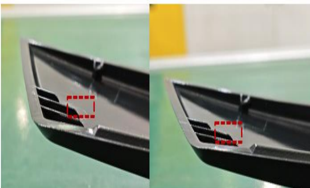
Gambar 2. Part shortmold area rib Sumber: PT. XYZ
